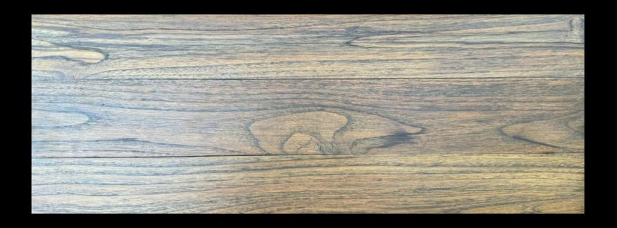
A smooth sanded floor is one in which the planks are made perfectly smooth with a flat floor surface and an even thickness.
